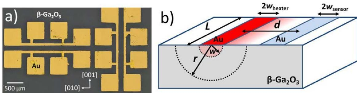
**Above.** a) An arrangement of two line heater pairs on top of the Mg-doped  $\beta$ -Ga<sub>2</sub>O<sub>3</sub>-crystal. b) The anisotropic thermal conductivity measurement setup to measure the temperature  $\Delta T$  between two metal lines (Au) through the  $\beta$ -Ga<sub>2</sub>O<sub>3</sub>-crystal with a thickness of  $t = 0.5$  mm.
